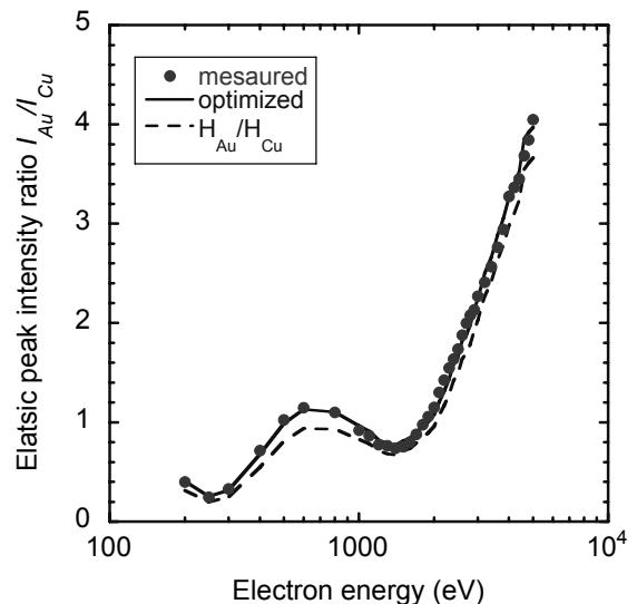
Fig. 3. Calculated elastic peak intensity (EPI) ratios  $I_{Au}/I_{Cu}$ , for Au to Cu with Monte Carlo calculations as a function of primary electron energies. The solid line shows the results of optimization with the proposed method and solid circles show the measured peak intensity ratios. The dotted line indicates the EPIs without surface-electronic excitation correction factor.
