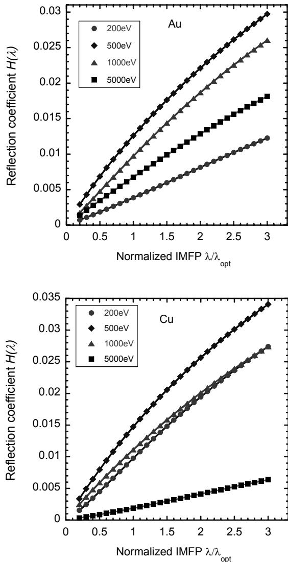
Fig. 2. Dependence of the theoretical reflection coefficient  $H(\lambda)$  on the normalized IMFPs for Au and Cu at several energies. Solid marks show the calculated reflection coefficient at several electron energies by MC method. The solid lines show the
