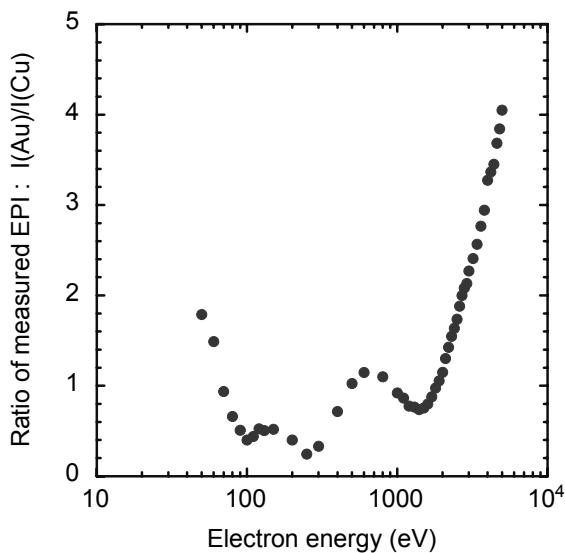
Fig. 1. Ratios of measured elastic peak intensities for Au to Cu as a function of primary electron energy.
