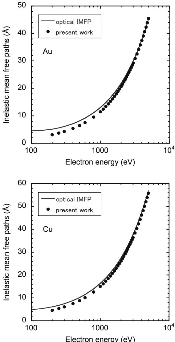
Fig. 4. IMFP values (solid circles) for Au and Cu determined from elastic peak intensity ratios in Fig. 3 as a function of electron energy. The solid line shows IMFPs calculated from Penn
